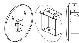
Case Style: Flush Movement Types: SS-24V, SS-120V or SS-WIFI Wall Box: 143 Install the 143 wall box (ordered separately) flush with the wall surface. Box dimensions are 6.5" x 7" x 3.25". 10" clock D=2.0"; 12" clock D=3.25"; 16" clock D=4.75"
