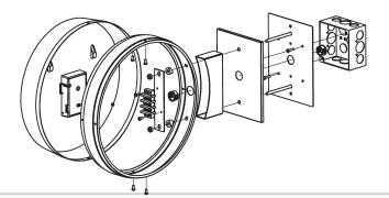
Case Style: Double Face Movement Types: SS-24V, SS-120V or SS-WIFI Wall Box: 4 Square Electrical Box (by others)
