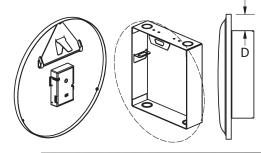
Case Style: 12" Flush Movement Types: SS-24V ,SS-120V or SS-WIFI Wall Box: Simplex, IBM, Lathem, Faraday, Edwards, Standard etc. The optional FR-12ADAPT-ST will provide the single-tang mounting compatible with other manufacturers wall boxes. 12" clock D=1.75"
