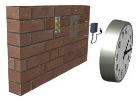
LEFT: Use the Wall Transformer (WT) version when power is from an existing outlet behind or near the clock location. Wire exit on top or bottom of clock if necessary.
